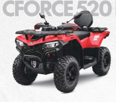
The 495cc engine of the CFORCE 520 adds more power and more possibilities to the agile ATV platform. Fortified with EPS, bigger torque and premium accessories such as RIDEVISION ® LED lights, aluminum alloy wheels, and 25-inch AT tires bring its rugged capability to a new level.
